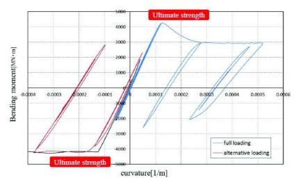
Figure 1.6 Repeated progressive collapse behaviour of bulk carrier in extreme sea [6].
