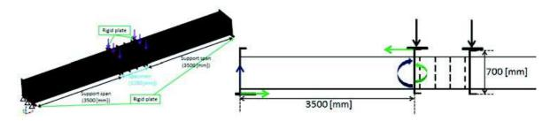
Figure 2 The schematic view for explanation of added bending moment induced by friction forces.
