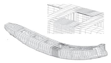
Figure 1.7 Sagging collapse mode in homogeneous loading condition [6].
