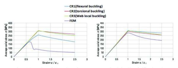
Figure 4 Comparison of CSR and FEM in stress-average strain relationships of stiffened panel
