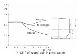
Figure 1.1 Progressive collapse behaviour of cross-section (double-hull oil tanker) [1].
