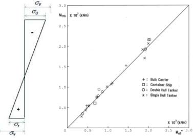
(a) Assumed stress distribution (b) Accuracy of estimated ultimate hull girder strength [2]
