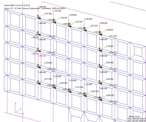
Figure 25: Particular of the coarse mesh model and displacements collected for application to the boundaries of the intermediate model.
