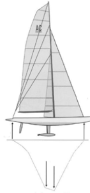
Figure 3: Bending moment diagram for an America's Cup Class yacht (Larsson, 2007).
