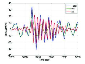
Figure 2. Stress measurements amidships on a large container vessel in a high sea-state. Direct wave-induced stresses on the rigid hull (WF), slamming-induced whipping stresses (HF) and the total combined stress, Andersen (2014).
